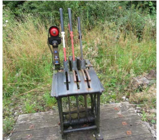
A manual control frame and interlocking controls at the west end of Bolton Abbey station
