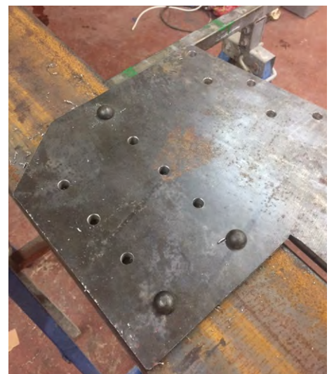
Riveting side plates
